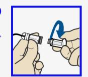
Twist the plunger counter-clockwise to loosen and remove.
