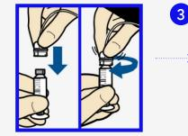
Gently push the tubing connector onto reservoir. Turn clockwise until locked. You will hear a click.
