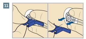
Hold infusion set. Pull **blue** handle straight out to remove needle.
