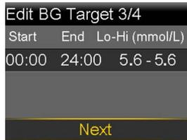
22) Press **^** or **v** to enter the **Hi** target and press **o**.
