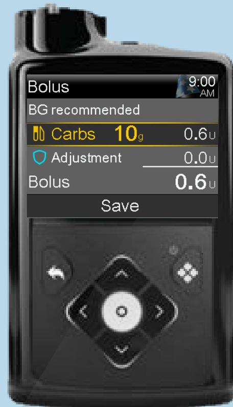
The **BG recommended message** indicates that the system recommends taking a BG for the Bolus screen to calculate a correction bolus amount.
