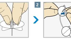
Peel off both pieces of the paper backing from the insertion piece.
