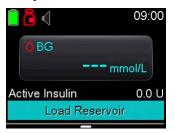
Press O to open the menu. If the pump is locked, you will need to unlock the pump after pressing O.
