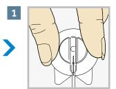
Hold infusion set insertion piece by flipping the plastic wings upwards and pressing them together.
