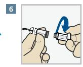
Twist plunger counterclockwise to loosen and remove.
