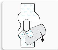
4. Rotate the 2nd tape and place the tape over the transmitter. Press it down firmly.
