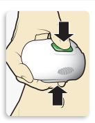
5b Insert the sensor. Press and release the **bump** on both buttons at the same time. Do not pull the serter away from your body just yet.
