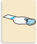
Remove the adhesive pad liner.
