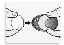
When you remove the transmitter from the charger, a green light should flash on the transmitter. This indicates that the transmitter has enough battery power to be connected to the sensor. If you do not see the green light flash on the transmitter, place the transmitter back on the charger until it is fully charged.
